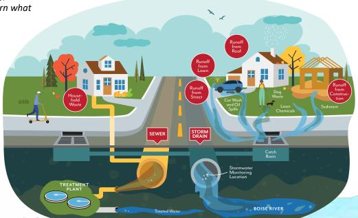
Most often, stormwater runoff from rooftops, yards, sidewalks, and streets flow into underground pipes through grates in the roadway.
