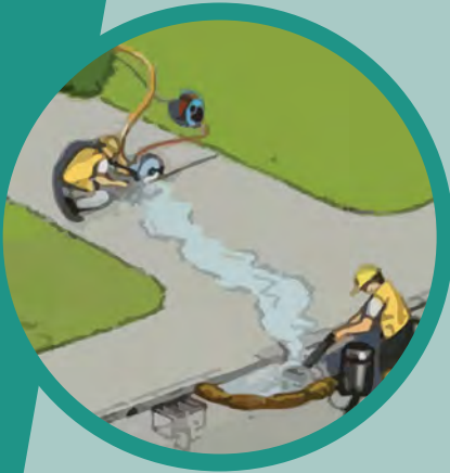
Concrete Cutting Slurry Containment and Collection
