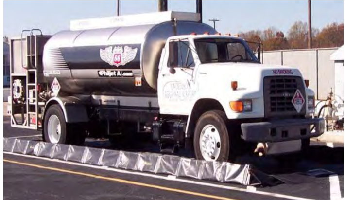
Figure 196. Mobile fueling truck (ITD 2014).
